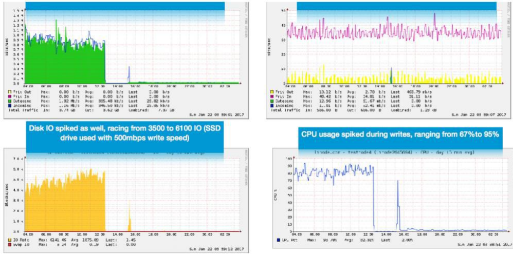
Figure 5.5.1 Part of the pressure test data result. Testing environment is using the lowest cloud server configuration in different locations worldwide. The configuration is 2G Single-core CPU/4G Memory.
