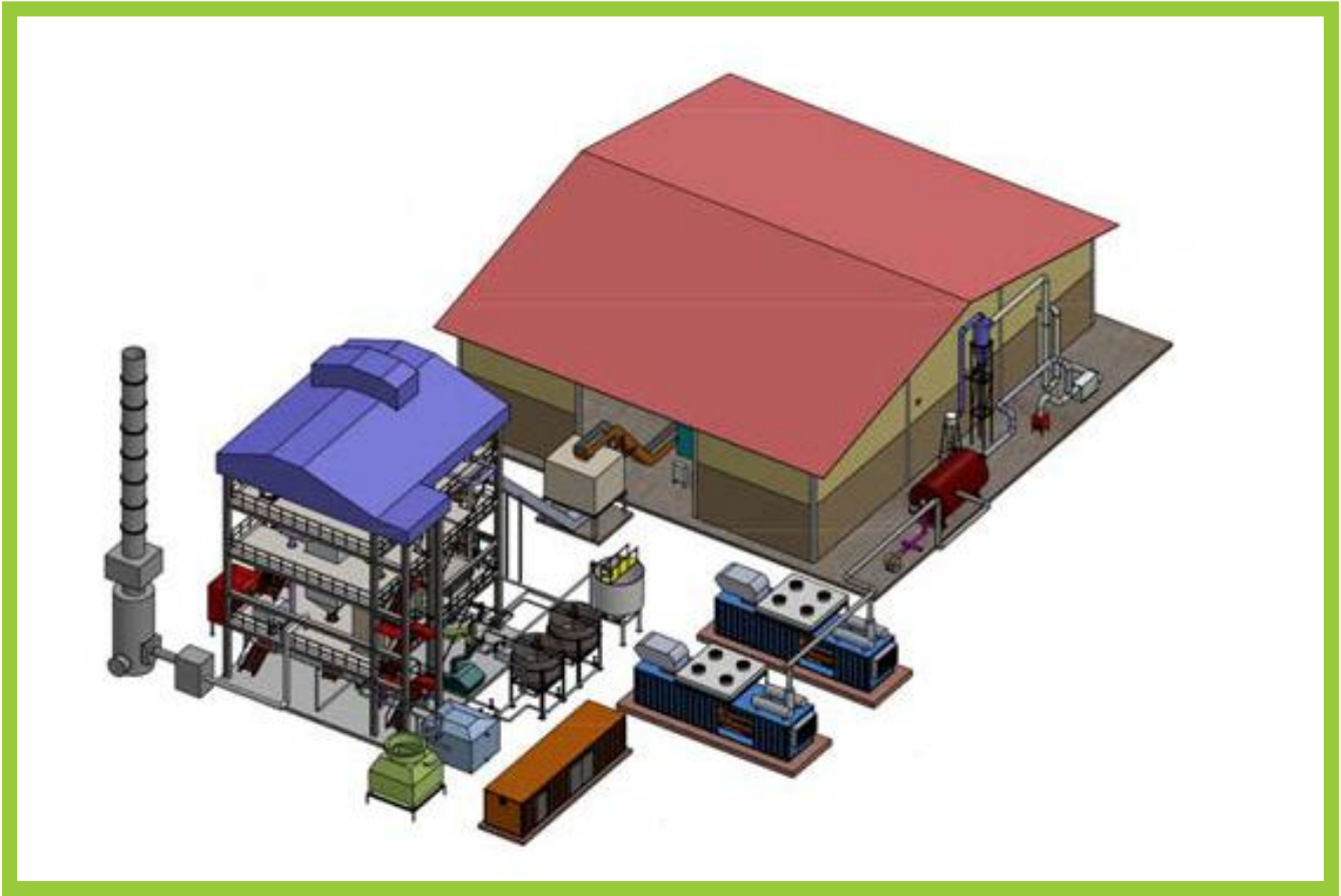
Figure 02: Complete Fluidised Bed Biomass Gasification Power Plant
