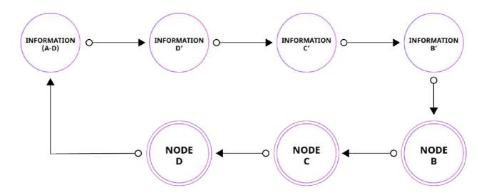
Unless Node B and Node C are controlled at the same time, it is almost impossible to know that Node A is sending a message to Node D.
