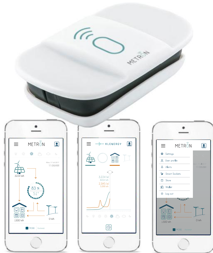
Figure 2: Metron Energy Monitoring System App & device
