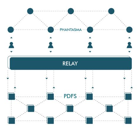
The Relay will operate running on top of UDP protocol, since it is a simple and effective low-cost protocol. It does not require the establishment of a constant connection, nor a guarantee of message delivery. These are features fit for fast data delivery to multiple recipients, and specifically useful for peer to peer applications - as is the case of the Phantasma Relay. The full specifications for the Relay's protocol will be detailed in a separate technical document.
