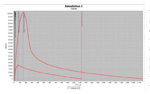
When we look at the rocket's Elevation and Time graph, two curves appear. One of them is the curve of the first piece fired first, and the other is the curve of the second and third stage. Two curves were formed because it showed the second and third levels as a single level and had their graph plotted in a single curve.
