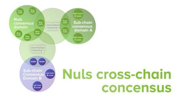
Main-chain consensus domain (surrounded by nodes of main-chain) Sub-chain A consensus domain (surrounded by nodes of chain A) Sub-chain B consensus domain (surrounded by nodes of chain B) overlapped /connected area: Cross-chain consensus domain A, cross-chain consensus domain B
