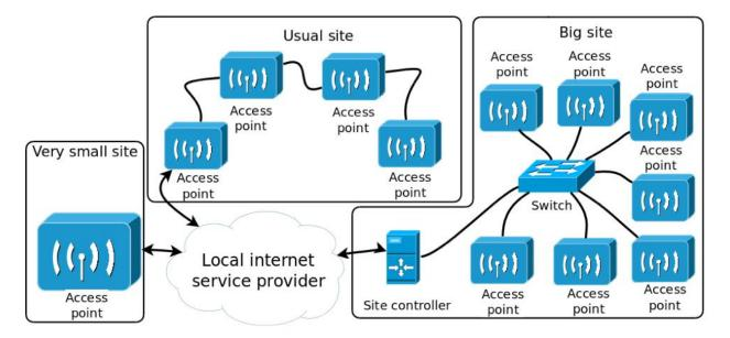
In very small sites off the shelf wireless routers running IUNGO provided custom firmware will be directly connected to local internet service provider. A selected set of the wireless router models will be supported by custom firmware to act as IUNGO network compatible access points. For
