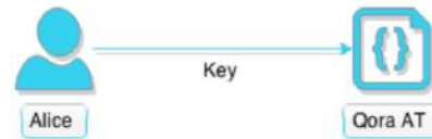
Figure 17. Burst/Qora ACCT step 3: Alice sends after examining the AT from Bob, the key to the Qora AT.
