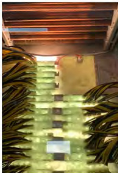
Fig. 8 Self-developed immersion cooling system
